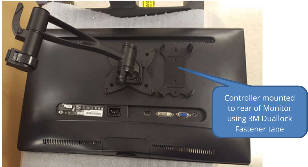
Figure 6: Attach Controller Mounting Clip to the rear of the Monitor
