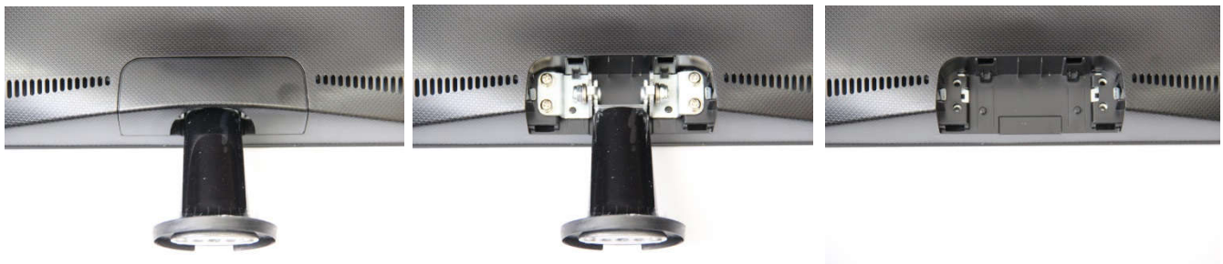
Figure 5 - Remove Stand from Monitor
