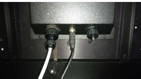
**Figure 20 - Insert Power Connector**
