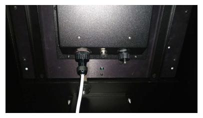
Figure 19 - Watertight Connection
