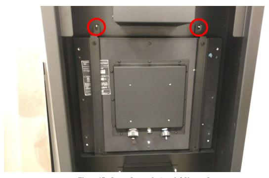
Figure 17 - Straps Inserted. Attach 2 Nuts to Secure
